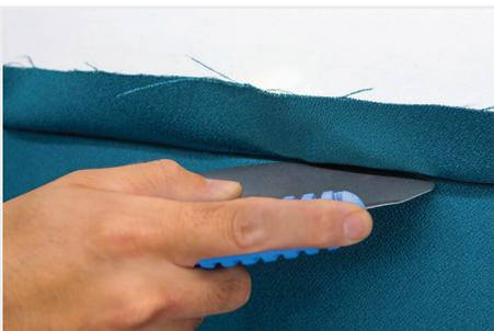
Now, starting from the top-center moving towards the corners, use the Rocker or Roller Tool to fully tuck the Fabric into the Frame jaws. Make sure to keep the Fabric straight during this process.
