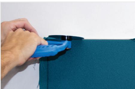
**Use Corner or Rocker Tool to tuck in corners first.** Then use Roller Tool to roll the remainder of Fabric into the frame jaws, hiding the excess. Very gently lean Roller Tool to the sides of the jaws while rolling for better results.
