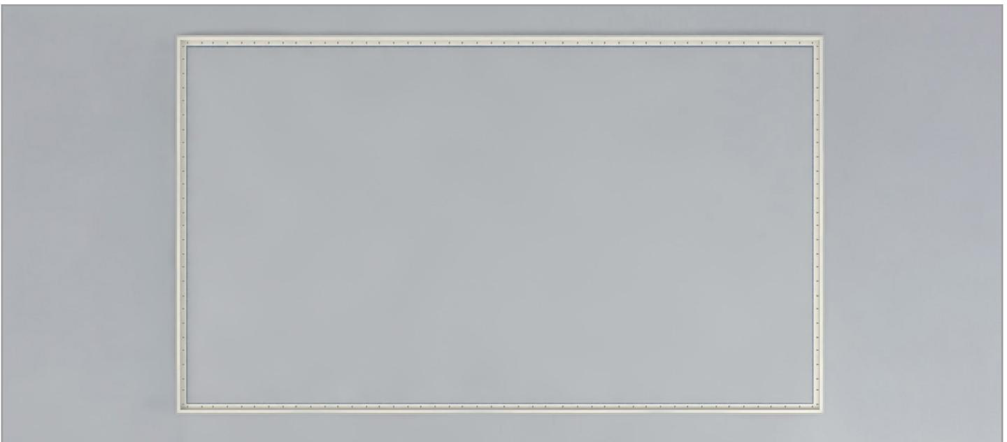
Staple or screw Frame to wall by placing staples every 1/2" to 1" or using screws every 5" to 6"
