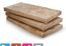
**Roxul** is a mineral wool or rock wool. It is forged with basalt rock and slag using a process in which they are superheated and their fibers are then non-directionally bound to create a resistant acoustical substrate. As heat is utilized in the process it gives Roxul excellent heat resistance of temperatures up to 2,150 degrees Fahrenheit.
