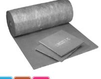
Flame-attenuated glass fibers give the Linacoustic® RC core notably better acoustical and thermal properties than other leading liners. This makes it more economical to use because the same or better performance can be obtained with a thinner liner. Linacoustic® is made from 100% Glass Fibers, supplies Superior Thermal Performance, and has an NRC of 0.55.
