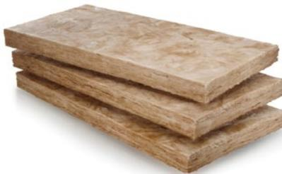
**Roxul** is a mineral wool or rock wool. It is forged with basalt rock and slag using a process in which they are superheated and their fibers are then non-directionally bound to create a resistant acoustical substrate. As heat is utilized in the process it gives Roxul excellent heat resistance of temperatures up to 2,150 degrees Fahrenheit.
