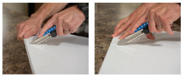
Use a Utility Knife to cut the Backing to size so it sits in the Frame flush and can be covered by the Fabric.
