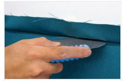
Now, starting from the top-center moving towards the corners, use the Rocker or Roller Tool to fully tuck the Fabric into the Frame jaws. Make sure to keep the Fabric straight during this process.
