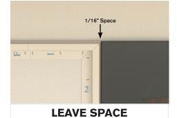
When working with FS100 or FS150 Frame, leave a small gap (approximately 1/16") between the Frame and the item it butts up against. This gap will allow the jaw to open when you roll in the Fabric.
